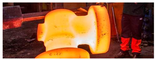
Riganti, founded in 1891, is a closed die forging master by mean of counterblow hammers, combining the flexibility of a craftsmanlike production with a state of the art technological know-how of a modern manufacturing enterprise.
