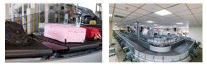
Fives customizes Baggage Handling Systems and provides advanced technologies to fully automate airport logistics by integrating circular cross-belt sorters, conveyors and carousels to transport luggage from check-in, HBS and EBS to final sortation and reclaiming.
